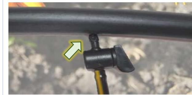
7. Insert 6mm Tap Valve in 16mm line & connect 4mm feeder line to desired length
