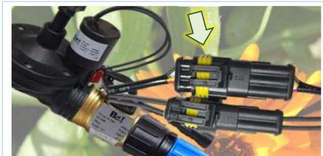
10. Plug in Sensor & Valve Electrical Pins to one end of Wire connecting Controller
